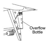
**NOTE:** If coolant must be added often, or if the overflow bottle runs completely dry, there may be a leak in the system. Have the cooling system inspected by your Polaris dealer.
